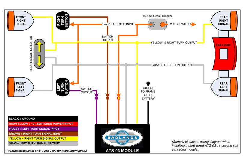
The wire colors in the drawing are used for reference only based on the colors we use on our module. When installing the hard-wired ATS-03 on a factory model, be sure to consult your bikes service manual for exact wiring diagrams and color descriptions to achieve proper installation.
