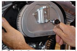
1. Refer to the service manual and remove the OEM air filter cover and filter element. The hoses will be re used.
