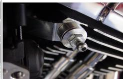
3. Re-install the breather bolts placing the the spacers over the induction supported bracket and the cylinder head.
