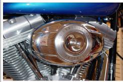
9. Remove the outer gasket from the OEM filter cover and install the cover with the OEM bolt.
