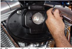
2. Remove the breather backing plate. The 2 breather bolts will be re used.
