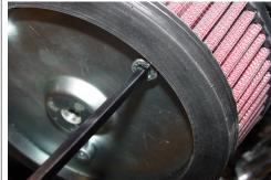
6. Install and tighten the filter element with the hoses onto the throttle body using the provided 1/4-20 X 2-1/2 inch bolts and new gasket.
