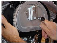
1. Refer to the service manual 2. Remove the breather and remove the OEM air filter backing plate. The 2 breather cover and filter element. The bolts will be re used. hoses will be re used.
