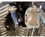
3. Attach the supplied support 4. Trim 5/16" off of each hose. brackets to the cylinder heads using the OEM breather bolts. Install the spacers between the bracket and the cylinder head. Do not tighten at this time.
