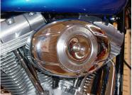
11. Remove the outer gasket from the OEM filter cover and install the cover with the OEM bolt.
