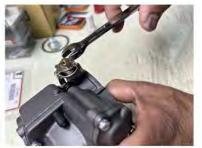
REMOVE NUT FROM LEFT SIDE AND APPLY LOCTITE ONTO THREADED BOLT AS SHOWN. FASTEN NUT BACK ONTO BOLT AND MAKE SNUG \*DO NOT OVER TIGHTEN\*
