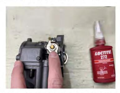
WE SUGGEST REMOVING THESE NUTS & APPLYING LOCTITE TO ENSURE THEY DO NOT COME LOOSE.
