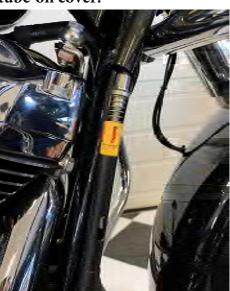
16. After you slide the cover on, reinstall the frame clips.
