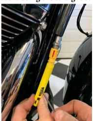
8. Remove the yellow plastic piece by spreading open the two small tabs on each side.
