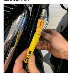
4. Use a straight screwdriver to remove the red clip. Then collapse the adjustor.
