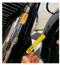
5. Rotate the yellow tube, and locate the little tab. Then separate it from the lower cable using the straight screwdriver.
