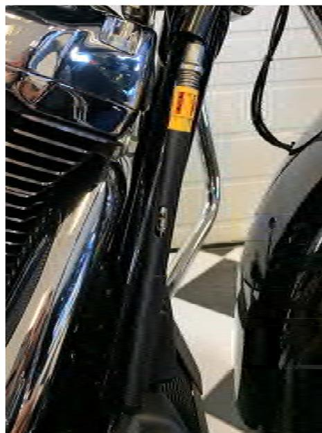
**15. Now you can adjust the clutch back cable and reinstall the black tube on cover.**
