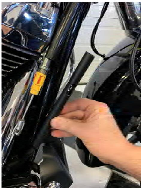
13. Push the upper clutch cable up the frame, and re-install into the new clutch extension tube.
