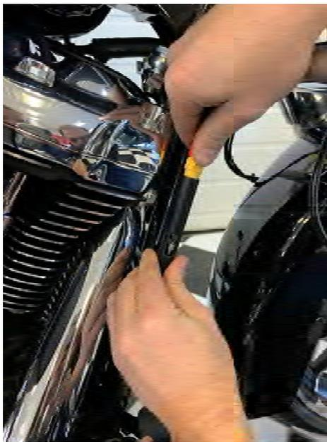
14. Connect the upper cable to the lower cable, through the oval opening in the black tube.
