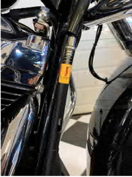
**16. After you slide the cover on, reinstall the frame clips.**
