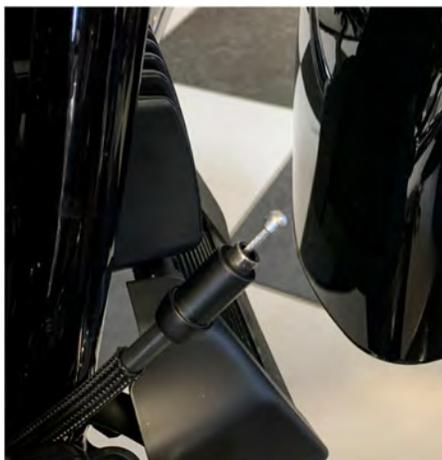
11. Use the two wrenches to loosen the adjuster on the wire extension. Slip the wire extension over the wire, hand tighten the nuts, bring the adjuster nut down, then tighten with the wrenches.
