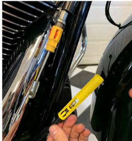
**8. Remove the yellow plastic piece by spreading open the two small tabs on each side.**
