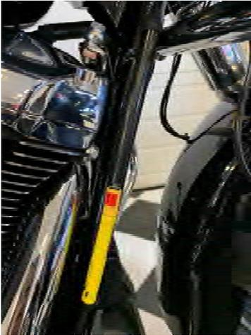
**4. Use a straight screwdriver to remove the red clip. Then collapse the adjuster.**
