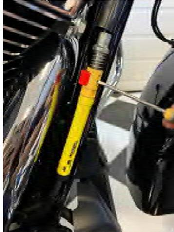
**5. Rotate the yellow tube, and locate the little tab. Then separate it from the lower cable using the straight screwdriver.**
