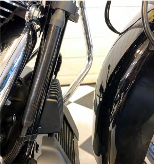
**2. Remove the cable clips from the frame. They will be reused.**
