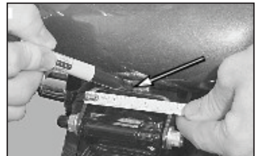
Figure 3. Mark the Fuel Tank Centerline
