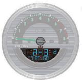
In the backlight (TAC) color (day) settings main screen, hold the button for 3 seconds to enter into the settings screen.
