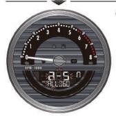
In the backlight (ALL: LCD+TAC+DIA) color (night) settings main screen, hold the button for 3 seconds to enter into the settings screen.
