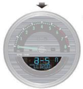
•EX: The backlight (LCD) color (night) setting is changed from 160 to 200.
