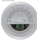
Hold the button for 3 seconds to move the cursor to the desired settings level.
