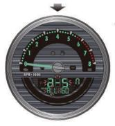
Press the button once to enter the backlight (LCD) color (night) settings main screen.
