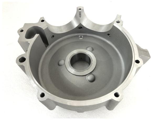
THE DEPTH OF THE FLYWHEEL SIDE MAY NEED TO BE INCREASED. MEASUREMENT FROM CENTER CRANKCASE JOINT SEEM DOWNWARD SHOULD REACH A DEPH OF 2.400. AREA NEAREST THE OIL SCRAPER NEEDS THE MOST MATERIAL REMOVED.
