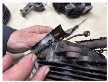
Adjusting form of oil lines may be necessary.
