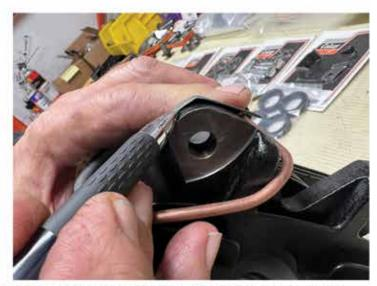
Check height of ears to ensure you have proper clearance. If clearance is an issue you must hand dress each rocker shaft ear for a proper fit.
