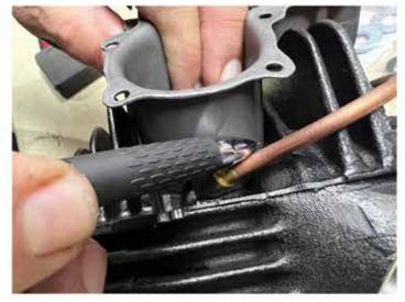
Ensure bottom of tin does not make contact with fins. If any areas make contact dress as needed.
