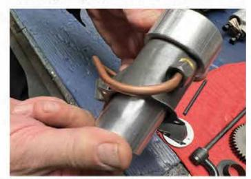
Insert male end of tool into female end encompassing irregular area of lower tin.
