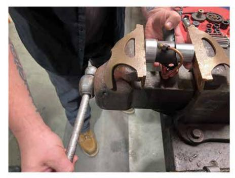
Place assmbled tool and lower tin into vice in a centralized location. Tighten vice firmly. Process could also be performed in a press.
