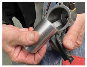
Place longer end of tool down into valve spring area of lower tins.
