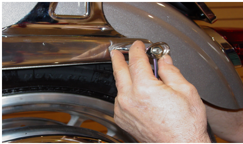
4. Align the side plated slot over the turn signal wire and re install the bolts in the turn signal assembly and front fender strut.
