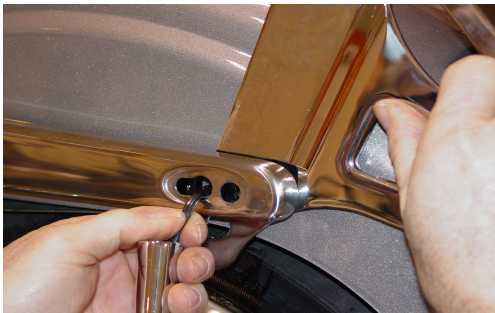
4. Align the side plated slot over the turn signal wire and re install the bolts in the turn signal assembly and front fender strut.
