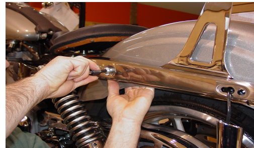
5. Re install the turn signal and fender hardware.
