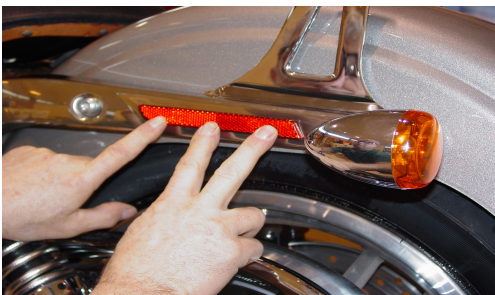
6. Install the reflector, using the provided tape.
