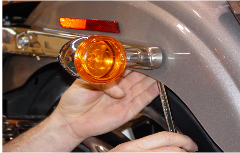
2. Remove the OEM turn signal assembly by removing bolt from under the fender
