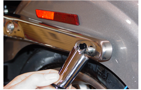
2. Remove the OEM turn signal assembly by removing bolt from under the fender
