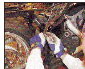
5. Mark fender struts and cut off. Both sides at the same angle. You can re-use these later.
