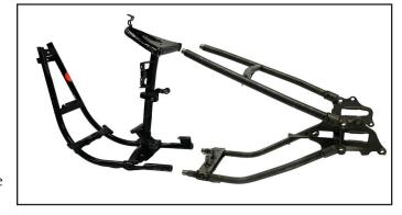
Once plate is mounted and frame plugs are inserted, they would then weld the frames together.
