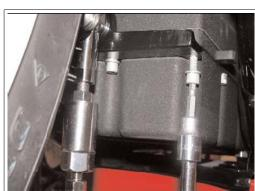
7. Install the bracket using the new bolts and washers. Torque to 10 ft-lbs.
