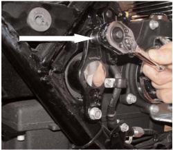
2. Remove the top bolt on the Swing Arm side plate only.
