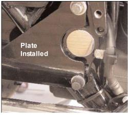
4. Remove the lower Swing arm side plate bolt, align the plate and a new washer and bolt. Torque both bolts to 35-42 ft-lbs.
