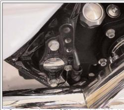
1. On motorcycles with OEM exhaust the right side exhaust pipes must be removed to access and remove the lower bolt on the swing arm side plate. Check to see if you need to loosen or remove the right side exhaust on your bike. If necessary accomplish this first
