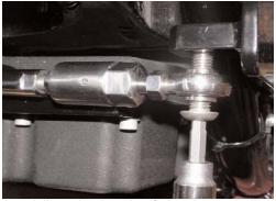
button head bolt. The strut has a left and right hand thread to allow adjustment of equal length.
