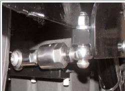
8. Adjust the length of the strut to allow 9. Tighten and secure the bolt with the proper alignment and install the provided 3/8 provided washer and nylock nut and tighten the jam nuts on strut.
