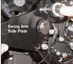
3. Place the supplied plate, washer and bolt as shown and start the bolt most of the way
