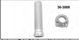
Anderson Twist Grip Assembly includes die cast housing with billet throttle tube with knurled surface. Note cables required. Accepts standard set.
