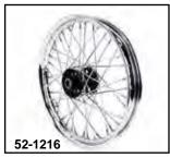
18" Replica Wheels with KH Type Rims. Fully assembled with a complete black star hub.
