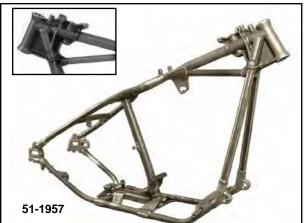
Replica Retro Rigid Frame features original style construction including forged parts in neck, side car mounts and rear axle areas. 103/4" between the rear axle plate. Order rear mount for TC-88 models separately.
