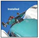
Chrome Fender Mount License Plate Bracket Kit includes a rubber anti-vibration block to cushion it against fender. Replaces stock three piece unit, bolts to same three holes, and uses light from stock tail lamp.
