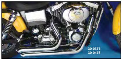
2¼" Drag Pipes fit FXD-FXDWG. Brackets are included. Order baffle rings separately.
