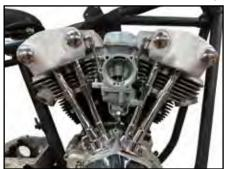
Retro Knuck Rocker Box Set for Shovelheads. Main body is supplied in casting is lightly polished.
