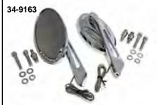
Billet Mirror Set features sequential LED turn signal on back side.
