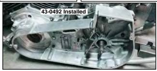
Cast FXE-FLH Inner Primary Cover Assembly for 4-Speed models.
