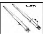
Fork Tube and Slider Assembly is available in right and left pairs, and is completely assembled. Units have hard chrome fork tubes, and either polished or chrome lower sliders, with springs and all internal components installed.
