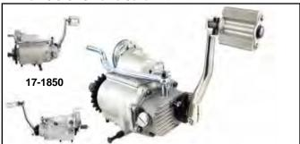
Sifton Kick Cover Kit includes a finned cover in a natural finish, with a stroker S.S. kicker arm, a black spring & a tempered tool steel kick shaft.
