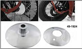
Spring Fork Hubcap Kit for 1936-48 Big Twins and 1957-59 Servi-Car. Kit includes right side "Atlas" chrome hubcap and left side chrome mini hub. Right hubcap has built in axle spacer and left side hubcap is held in place by wheel hub seal spring
