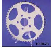
**5-Spoke Sprockets.** Offset models have 9.8mm offset. Offset type fits 1973-84 FX, FL and 1979-81 XL rear hubs. Flat type is for custom applications.
