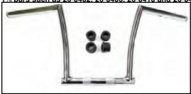
**ChiZeled Chrome Handlebar.** Notched for throttle by wire applications and slotted for internal wiring.
