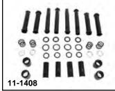
M-8 Adjustable Pushrod Conversion Kit includes chrome covers, adjustable pushrod set and o-rings. These pushrods are tapered for enhanced clearance at the cylinder head, allowing the use of higher lift cams. The one-piece chrome moly pushrod adds rigidity and durability and the threaded adjustment feature provides easy cam installation without removing the cylinder heads or rocker boxes.
