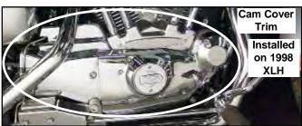
Form Fitting Chrome Steel Covers fit over stock cam cases on XL models. No need to remove cam case or disturb cams or gears. Covers held in place by existing screws and related hardware as supplied. Note: 42-9962 is kickstart only. All other numbers are for electric start.
