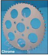
**1973-84 Big Twin, 1979-81 XL Rear Sprockets**. Replace OEM 41470-73. Used on all 1973-86 FX, FXE, FXEF, FXWG, FXST, FL and FLH, 1979-81 Classic, cast or wire wheel. Dish type sprocket with 9.8 mm offset.
