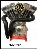
53/4" Chrome Air Cleaners are for 3 bolt carburetors. Includes foam washable element. 21/4" thick.
