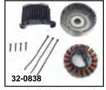
Alternator Kit for FLT models include rotor, regulator, stator and hardware. Use 32-8926 or 32-0746 rotor only with 32-7780 kit, to produce 45 amp output.
