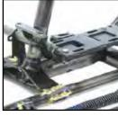
**Rear Engine and Front** Transmission Mount is of forged steel, with bushing installed. Transmission mounts incorporate a formed reinforcement strap to connect the two tier support strap assembly, all of which is constructed accurately of blanked and formed stampings.
