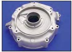
Moto Shop Alternator Sealing Ring Replacement Service. Ship in 1970-up left hand case with damaged O-Ring lip and we will machine out and replace with new steel sealing ring.
