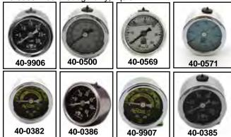
Liquid Filled 11/2" Oil Pressure Gauges feature weather resistant sealed lens, stainless steel case, chrome rim and extra heavy mechanism. Liquid filled face eliminates needle bounce giving a constant reading. All gauges have 1/8" NPT male rear fitting.
