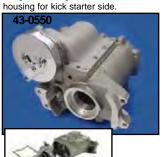
4 Speed Transmission Case and Ratchet Top Set fits 1965-Early 1979 Big Twin. Both parts are in a natural alloy finish. Case accepts Torrington 4th gear bearing VT No. 12-0300. FLH style ratchet top gives 1 down, 3 up shift pattern and is assembled with all internal parts, including chrome dust cover and arm.
