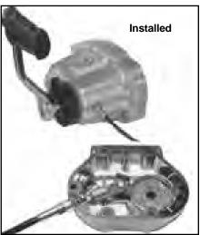
**E-Z Pull Clutch Assist** reduces manual effort required to pull the clutch lever by 40%. Mechanism fits inside transmission side cover and extends clutch operating mechanism for improved leverage.
