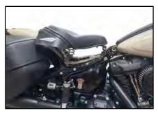
2018-up ST Solo Seat Mount Kit a steel frame cover plate, which incorporates the solo seat lower spring perch.
