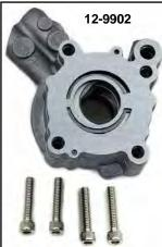
**Twin Cam Super Pump** by Sifton utilizes an oversized highly efficient Geo Rotor design. Provides a 40% increase in pump volume and a 60% more scavenging volume. This high volume pump bolts into the stock location and includes O-Rings and mounting hardware.
