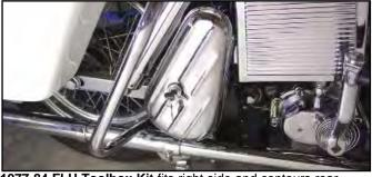
**1977-84 FLH Toolbox Kit** fits right side and contours rear shock and bolts to rear battery tray and exhaust tube mount. Kit allows use of FXE or FLH exhaust.
