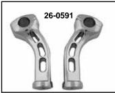
Chrome Pullback Riser Set features pullback styling. Kit includes two piece cap set and risers with 5" rise and 2" pull back and ½" — 13 internal threads.
