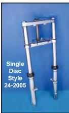
FXST 11.5" Single Disc Style Fork Assembly fits FXR 1982-94 or 1991-up FXD Dynaglide models. Assembly is available with chrome triple trees, polished or chrome lower legs without reflector boss to accept a left side single disc 1984-99 type caliper and 111/2" brake disc. Hard chrome fork tubes with internals assembled, axle, neck bearings, top cone, stem nut, pinch bolts and bearing dust covers are included. Stock unit is 31" overall length. FXR units do not include provision for fork lock.
