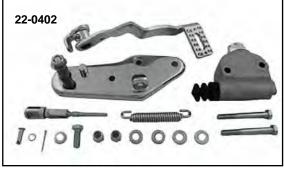
**1958-69 Hydraulic Brake Kit** includes all parts illustrated as replacement for flat side engine or for use on cone motors with an outside frame pipe.
