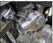
Carburetor Air Intake Snoot constructed of cast aluminum with a polished finish for S&S and shorty carburetor applications. Includes the carburetor air snoot door.
