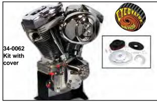
Cycovator Air Cleaner Kit fits 1999-up Big Twin with carburetor. High filtration element included with all parts as pictured. Order 34-1186 adapter sleeve to fit 1993-98 Evolution models.
