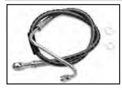
10mm Stainless Steel Banjo End Dual Disc Upper Hose fits 1982-up style master cylinders for single or dual disc application. Hose has nut with inverted flare at opposite end. The length from the banjo to the first bend is 24".
