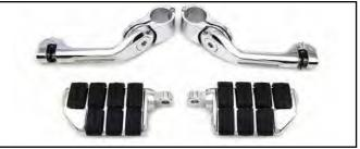
Highway Bar Kits clamp on 1¼" diameter tubes. VT No. 27-1013
