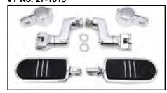
Chrome Streamliner Footpeg Kit includes rubber inlay set, offset footpeg mount kit, and clamp set. VT No. 27-0485
