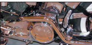
True Dual Chrome Exhaust Systems feature a single pipe for each side. Each pipe is independent and has 134" outside diameter. The rear pipe is for the left, and the front pipe is for the right without intersection.
