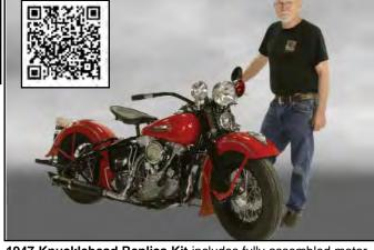
1947 Knucklehead Replica Kit includes fully assembled motor, transmission, wheel assemblies and fork. All parts included except paint and assembly. Restoration finish in black and parkerized. See web parts build list. Assembly by Tom Owejan.
