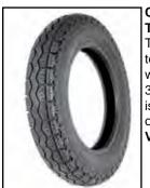
Coker 500 x 16" Treadwall Trackmaster is a tube type tire. Tire measures 25.75" in diameter and features a width of 4.75" when inflated on suggested 16 x 3" rim. The four-ply construction is authentic for most restorations of vintage motorcycles.
