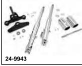
FLH Style Fork Assemblies are available as single disc model 1972-84 type, which accepts large banana caliper to accept a 10" brake disc. They include chrome slider covers, and chrome triple trees that accept aluminum cowlings and a lower tree that includes a padlock tab. Also included axle and nut, neck bearings, top nut, crown nut, sliders with stock length tubes and all 1977-up type internals installed.
