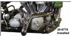
Wyatt Gatling Lake "Y" Dumper Exhaust Pipes feature 2" header pipe and a 3" collector end that turns out. Available with or without baffle. These are super loud. Will not fit with footboards. Fits 1986-up FXST, 1991-19 FXDWG.
