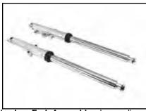
41mm Single Disc Leg Fork Assembly where caliper is on left side for 11" rotor.
