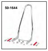
21" One Piece Rigid Mount Sissy Bars features a steel upright that is welded to the rigid mount side plates. Bolts directly to fender struts for a narrow profile and clean installation. Back rest pad is not available. **Note:** Installation hardware included.
