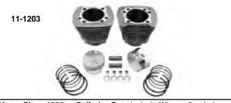
Motor Shop 1200cc Cylinder Sets include Wiseco fitted piston and ring sets to be used with 1200cc heads only. Fits 1988-03 1200cc as stock replacement on 1200cc only. Can not be used as Big Bore Kit for 883 models.
