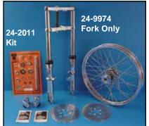
41mm Glide Fork Assemblies include forged chrome replica triple trees and hard chrome tubes on stock length forks, chrome tubes on overstock length and polished or chrome lower legs with all internals installed less hardware. Stock overall length is 31".
