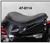
**Metro Solos** are covered with genuine leather on a stock formed steel ribbed baseplate with a rolled and sewn edge and black leather skirt decorated.
