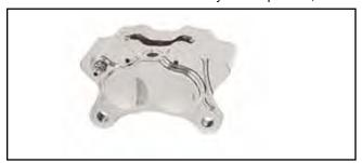
Chrome Four Piston Brake Caliper Kits are of the highest quality available. The piston are hard anodized aluminum for superior operation and long lift. Brake pad springs eliminate rattles and aid in caliper installation. Direct replacement for stock caliper and bracket. Use with stock brake controls. Require brake line fabrications by installer. Use with D.O.T. 5 brake fluid. Caliper mount holes are 3½" center to center.
