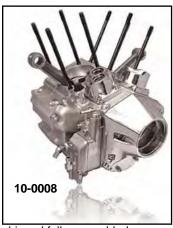
V-Twin™80" Short Blocks are shipped fully assembled as shown. All 80" units feature an S&S Crankcase, Sifton Oil Pump/Breather assembly, stock stroke flywheel, Timken Bearings, stock cam properly installed with a matched pinion and cam gear with Torrington bearing. Assembly is supplied with a chrome nose cone cover and chrome lifter blocks are fitted with standard tappets.
