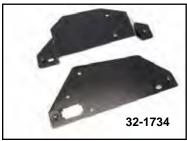
Black Electric Panels fits 1982-90 FXR. Flat left and offset right FXR electrical wiring panel set. Panels mount by 1/4"-20 well nuts and 1/4" x 20 x 3/4" screws.
