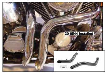
**Chrome LAF Exhaust Header Set** with a down style and features a 2½" diameter. Sold in a quantity of 2. Set is for left side and right side drive applications.
