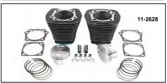
93.4" Cylinder Kit includes Wiseco 9.5:1 compression piston set with rings pre-fit to new 3.75" cylinders. Cases must be bored to accept this kit.
