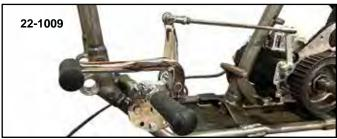
5-Speed FXST Replica Forward Shifter Kit is complete with all hardware necessary for installation on 1981-up 5-speed Big Twins. Use in conjunction with our FXST Replica Controls listed on the opposite page, as all kits place pegs in a forward position. Foot rests on peg while shifting for added comfort. This is an exact stock replacement in chrome for 1984-up FXST. Kit includes chrome heavy duty shifter bracket, inner lever, shifter lever, rod, rubber shift peg and foot peg.
