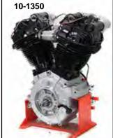
Complete Knucklehead Motor Assembly with Linkert Carb
