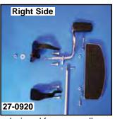
Wyatt's Footboard Kit for FXD is designed for use on all 1996-up FXD models. It features the same style used on all touring models to maximize rider comfort. The kit comes complete with footboards, mounts, brake pedal, extended brake rod and extended shifter rod and mounting hardware.
