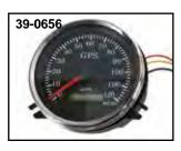
GPS Speedo and Speedo Tach Gauges mount to cast and steel dash panels. 1968-up cast, 2/3 light and cat eye types. Speedo is clamped to dash panel with speedo back clamp, fitted with rubber gasket to seal dash panel. After gauge rim is fitted to rubber gasket in dash panel, turn back clamp on speedo body to lock in position a direct bolt in to replace electronic speedometers. Includes back clamp and rubber seal and GPS satellite sensor. Sensor must be mounted on outside motorcycle signal.
