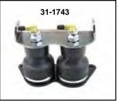
Solo Seat Air Shock & Seat Mount Kit includes a weld-on type rear mount and air cushion, for riders up to 175 pounds. VT No. Item
