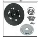
Pro-Lock Clutch Kit features a positive engaging ball ramp activation system, this applies extra pressure to the clutch plates and prevents clutch slippage without any increase on the lever pull effort by changing the fulcrum point. Fits straight into the stock clutch basket and behind the stock primary cover. Replaces stock pressure plate, diaphragm spring and spring retainer. Fits 1998-17 FXST, FLST and 1998-16 FLT.
