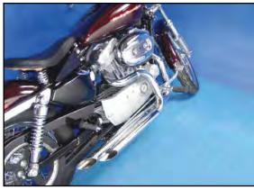
**2007-13 XL Side by Side Pipes** fit XL and XLC models with forward controls. Pipes are 1¾" at head and 2¼" at end and includes brackets and baffle set. 2007-up has provisions for oxygen sensors. Sensors may be capped by 30-0423 if desired.
