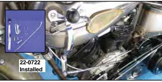
Chrome 4 Speed Ratchet Top Tank Shifter Kit features smooth gate, handle and rod and pivot bolt for 3.5 gallon tanks for years listed.
