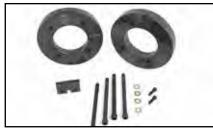
Jims M-8 Cylinder Torque Plates. Aluminum cylinders cannot be accurately honed and measured without the use of torque plates. The Jims Torque Plate kit for use on Milwaukee-Eight ® cylinders will simulate operating stress conditions when boring or honing cylinders. These plates adapt easily to conventional boring bars or Sunnen honing machine, and do not require the removal of ring dowels. Use on 2017-up Milwaukee Eight® engine
