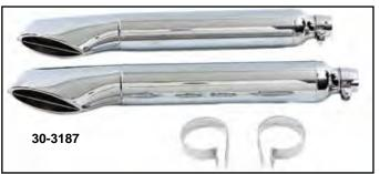
V-Twin™ Replica Chrome Seamless Muffler features classic fishtail or turnout ends with factory duplicated stock seams and welding for restoration or nostalgic looks with a 31/4" outside diameter. All fit 134" inlet, single and dual applications. Pairs include two mufflers and four clamps.
