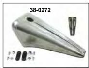
**Stretch Tank** features flat bottom for universal mounting on extended neck frames, 24" long. Right hand bung.
