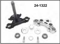
Triple Tree Set includes a polished aluminum cast top tree and a black steel lower tree.
