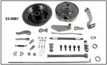
Rear Brake Drum Kits feature backing plate with all components installed, including a pre-arced set of brake shoes to fit the drum supplied. The drum has the 51 tooth sprocket riveted on with an original style dust ring. Kits are available in black or chrome finish. Lug bolts included, but axle and sleeve kit must be purchased separately.
