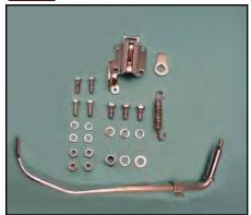
Chrome Kickstand Assembly fits 1936-85 models. Kit includes late style mount bracket with built in spring plate, lock tab, spring and flat bottomed forged side stand with mount hardware. VT No. 27-1720
