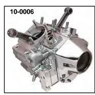
V-Twin™80"Short Block is shipped fully assembled as shown. 80" unit features a S&S Crankcase, Sifton Oil Pump/Breather assembly, stock stroke flywheel, Timken Bearings, stock cam properly installed with a matched pinion and cam gear with Torrington bearing. Assembly is supplied with a chrome nose cone cover and chrome lifter blocks are fitted with standard tappets. Block fits 1973-84 Shovelhead.
