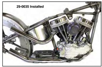
Upsweep Header Set will accept straight fishtail extensions or mufflers which must be purchased & mounted separately. Fits 1948-57 Rigid Frame Panhead Only with kickstart engines. Features 'S' type front pipe for better ground clearance.
