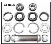
Rear Hub Rebuild contains all internal parts including longest length inner spacer (white 4.4480"). Spacer can be cut down or collar removed for some applications. Fits 1973-82 FL-FX. VT No. 44-0426
