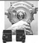
1990-98 Big Twin Snap Ring Remover will remove the Timken Bearing outer race snap ring without damage to the case VT No. 16-0705
