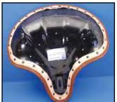
Corbin-Gentry Leather Solo and Buddy Saddles are built on a replica style steel ribbed baseplate with brackets riveted in place. Original style seams are accomplished by riveting a leather strip to the seat pan and form fitting the leather cover to strip and sewing for authentic construction.
