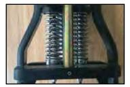
Chopper Style Springer Fork Assembly features 1-24 thread neck stem and rockers with a ¾" axle hole.
