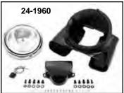
1960-84 FLH Headlamp Cowl Kit available with complete light assembly with rim and chrome or polished housing set with matching top handlebar cover as pictured.
