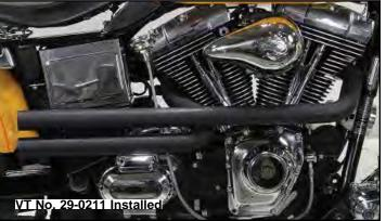
**FXD Shotgun Style Exhaust Drag Pipe Set.** Fits 1991-17. Pipe set has 18mm O² oxygen sensor bungs and includes plugs for non-EFI applications. 2012-17 applications will require separate purchase of **VT No. 32-6578**. Straight pipes may be fitted with mufflers or baffles, available separately.
