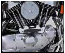
Chrome Tappet Base Cover is die cast one piece covering the area from the pushrod tube base to the cam cover. Fits 1991-2003.
