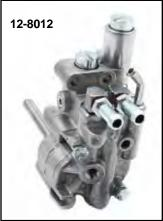
**Oil Pump Assembly** for Big Twins is high-quality replacement cast aluminum pump body with steel gears and shafts. Features cast aluminum finish. Gaskets and seals included. Mount hardware sold separately. **Note:** 1973-80 models may require drilling of crank case use drill jig **VT No. 16-0986.**
