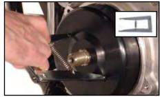
Big Twin Alternator Rotor Puller uses the two threaded holes in rotor to allow removal of rotor.
