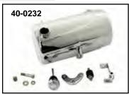
**Round Oil Tanks** fit 2000-17 Twin Cam-Softail models with center or side fill. Tank is 6.5" diameter, 11.75" long and requires removal of coil bracket and relocation of coil. Order mount kit separately. **Note:** Will not fit rocker models.
