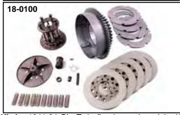
**Clutch Pack Kit** for 1941-84 Big Twin fits 4-speed models. Kit includes kick or electric clutch drum, 3 or 5 stud complete clutch hub, 4 steel and 5 fiber plates, clutch springs, outer clutch, releasing disc and clutch hub nut with lock tab, key and seal.
