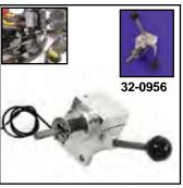
The Lever Starter System with stik start is made from CNC billet aluminum and assembled with accurate components. Unit fits 4 speed electric start models from 1965-88 with separate starter solenoid. This hand operated system will always work. It mounts in the place of the starter solenoid; just pull the lever and go. Requires separate purchase of starter relay depending on wiring configuration. See instructions on the web.
