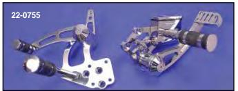
**Chrome Billet Forward Control Set** fits 1986-99 Softail, 1958-84 FX-FL includes rubber belted pegs as shown. Includes shifter and brake side with master cylinder. Order shifter rod and stainless steel brake lines separately.
