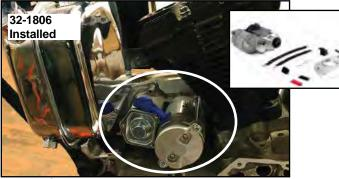
**Electric Starter Kit** includes a 1.4kw compact starter with integral Bendix, solenoid and gear reduction.
