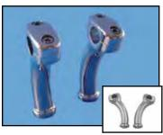
Chrome "Fatty" Curved Riser Set features pull back styling as on 2000-up models. Kit includes two piece cap set and risers with 5" rise and 2" pull back and ½" x 13 internal threads. Replaces 56033-00.
