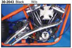
Note: Wyatt Gatling Exhaust Set features "Quad Finishing" which includes triple dura nickel and chrome as the final finish. After chrome plating, pipes are normalized and dried @572°F for the final finish process.
