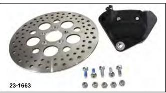
Front Caliper and Rotor Kit fits 2000-07 FXST models. Kit includes a complete replica 4-piston caliper assembly with pads, polished stainless steel drilled rotor and chrome mounting bolts.
