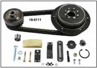
Primary Chain Drive Systems for Big Twins include 76 or 82 link Diamond primary chain, chain shoe adjuster assembly, clutch drum basket with starter ring gear and steel and fiber clutch plates with pressure plate assembly. Correct front compensator sprocket assembly includes all parts necessary for installation. Including sprocket nut. 5-Speed Big Twin Softail models and all pre1985 FLH-FX 4-Speeds require 82 link primary chains, 1980-up FLT-FXR 5-Speeds require 76 link primary chains.
