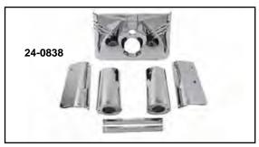
1986-17 FLST Complete Chrome Cover Kit includes front panel, left and right panel, upper slider covers and side trim strips.
