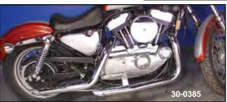
2¼" Drag Pipe Set features built in mount tabs to bolt to stock bracket. Chrome replacement bracket and baffle set available separately. Fits 1986-03 XL models.
