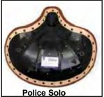
**Replica Dark Brown Leather Solo Seat** as installed on the "Fireman Bike." Base plate is vented type with holes. Order stock and custom mount kits separately.
