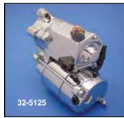
High Torque Starter Motor by Volt Tech are available with 1.4 kw field wound. Stock starter motor is 1.2 kw field wound type. Chrome units have all aluminum parts, polished and all steel parts chrome plated. All units are supplied with jackshaft bolt.
