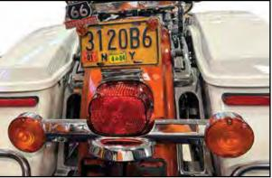
**License Plate Bracket** relocates plate to above tail lamp. Fits behind OEM tail lamps mounted on FLH fender. Fits 1980-up FLH, 1973-1984 FX.
