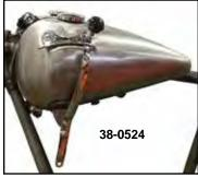
Fat Bob 3.5 Flatside Fat Bob Tank Set features handshift gate provisions to fit early style gates for 1936-46. These flat side tanks feature screw type bungs. Order caps separately. Petcock fitting should be masked or plugged during painting for easy installation. The side tank features side shift tank mounts. For use with cateye 1936-1946 type shifter gates or the conversion gate for 5 and 6 speed models, smooth type.
