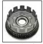
**Alternator Rotor Clutch Shell Assembly** feature vibration proof magnet construction, as magnets are held in place by stainless steel non-magnetic insert for durability. Replaces 36791-84. Fits 1984-90. Bearing and ring gear included.
