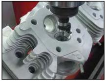
Motor Shop Ready Head Remanufacturing Service. Available as a valve job only or as a valve seat/valve job remanufacturing service. We will glass bead heads, install new cast iron guides, nitrated coated valves, spring, collars and keepers for both services. For valve seat service all of the above will be done with the addition of installing new no-lead valve seats. Heads must be in rebuildable condition and will be done in sets only. Service will be performed on a Sunnen Valve Machine.
