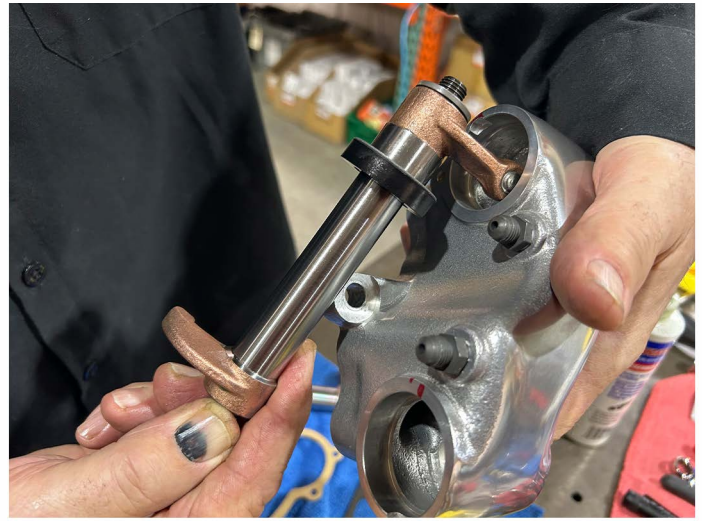
Rocker Arm shaft is slid back to allow one to turn or angle arm into box.
