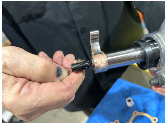
Close up of sealant being applied.
