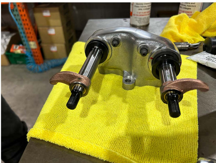
Rocker box assembly ready for seals to be pressed into position.
