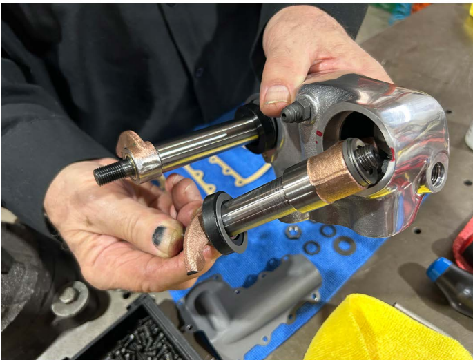
Again, said Rocker Arm is angled into its rocker box cavity with its respective shims,
