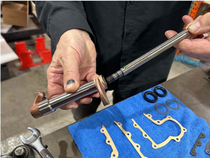
Insert Rocker Shaft into Rocker Arm itself.
