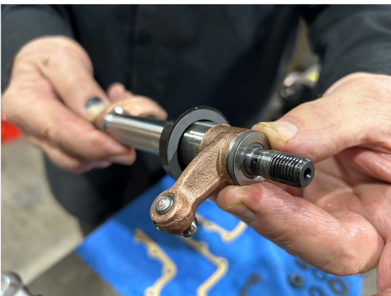
Outer view of Rocker Arm thrust washer with .007 shim installed over its respective lip. Its lip always faces the Rocker Box face inside to inhibit proper oiling.
