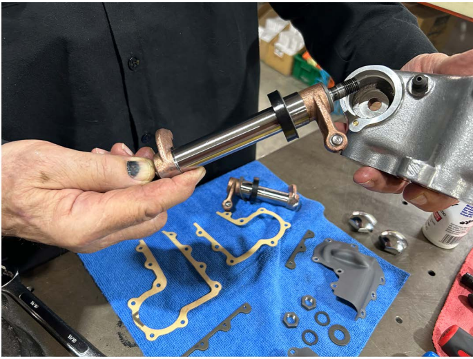
Rocker Arm ready to install into its respective Rocker Box position.
