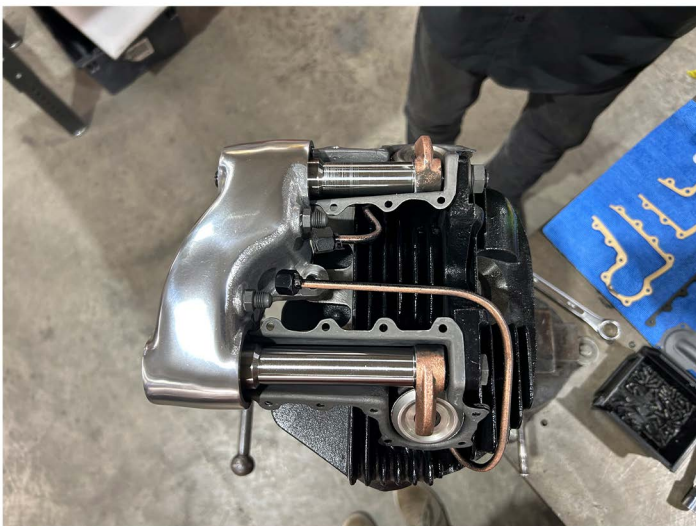
Top view of assembled rocker arms. Once fitted temporarily remove to properly apply sealant to tin covers.
