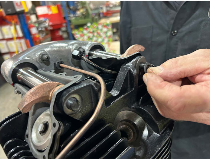
Front Intake shaft utilizes space in washer with lockwasher due to its long motor mount extension. Note that ONLY intake shafts require this additional washer. Exhaust shafts only utilize the lock washer.
