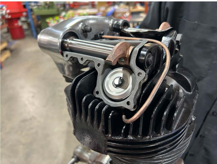
Front exhaust shaft lock washer in place.
