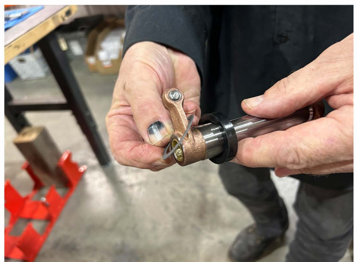
Follow said seal with proper installation of its support washer.
