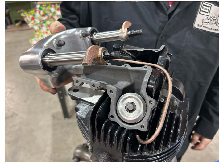
Front exhaust shaft nut installed with lock washer.
