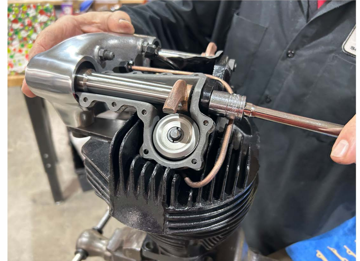
Tighten front exhaust proper!
