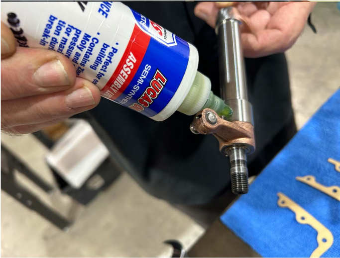
Apply assembly lube to rocker arm journal to inner seal surface.
