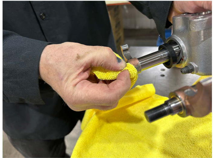
Prep each shaft end to receive sealant.
