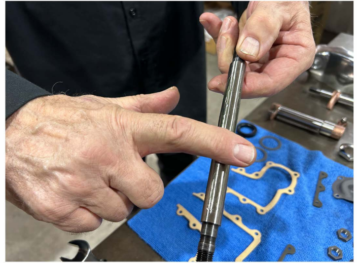
Initial assembly of Rocker Arms with Shafts. Note the proper use of assembly lube.
