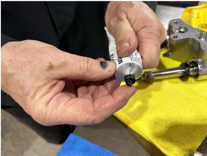
Apply a light film of sealant to left shaft end at cylinder head support bracket area only.
