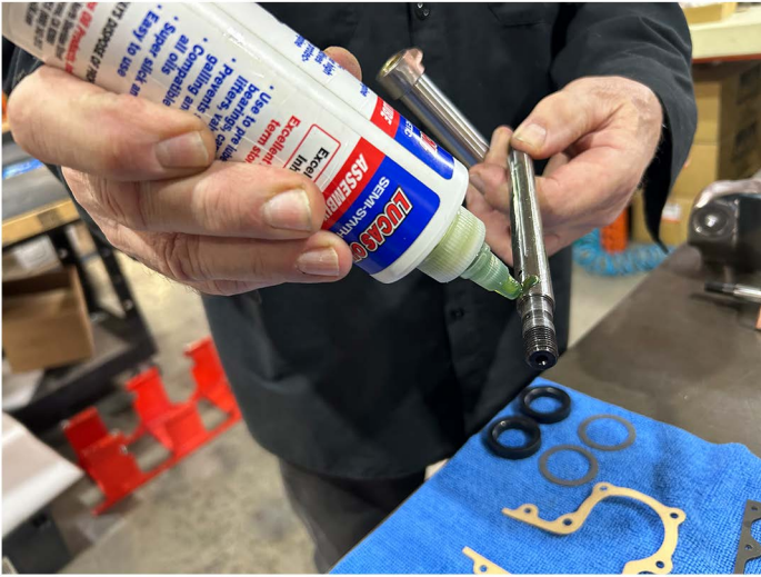
Initial assembly of Rocker Arms with Shafts. Note the proper use of assembly lube.
