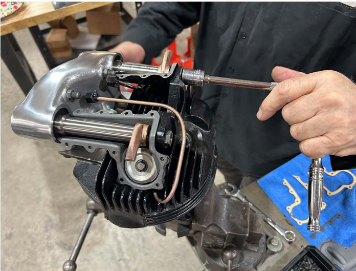
Now properly tighten each rocker shaft nut. Front intake shown.
