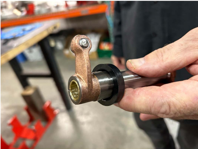
View of rubber seal on rocker arm journal with proper assembly lube.
