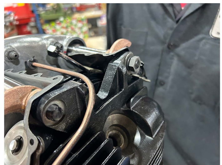
Front Intake shaft utilizes space in washer with lockwasher due to its long motor mount extension. Note that ONLY intake shafts require this additional washer. Exhaust shafts only utilize the lock washer.
