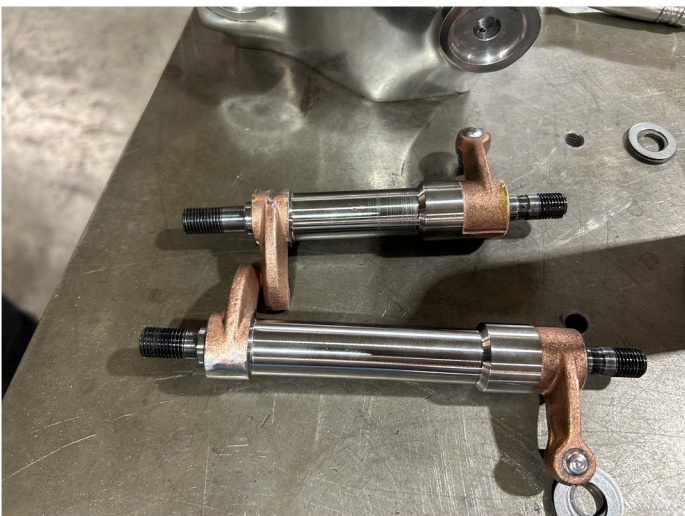
Rocker Arms and shafts ready for installation.
