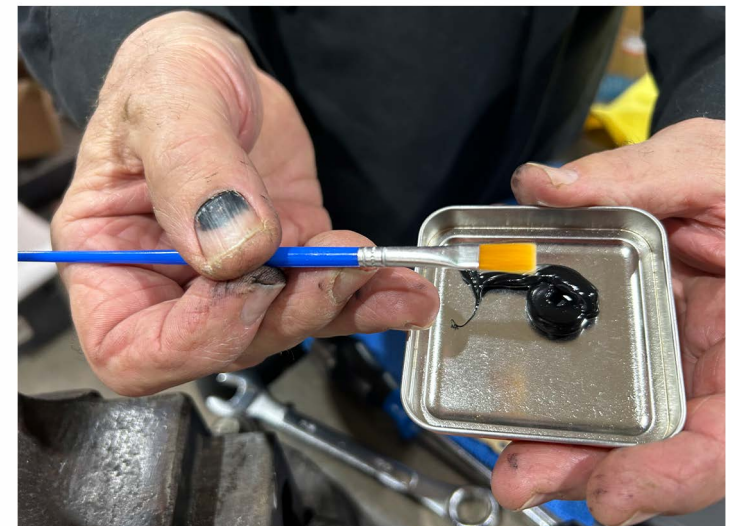
Prepare a small container to apply sealant with small brush as shown.
