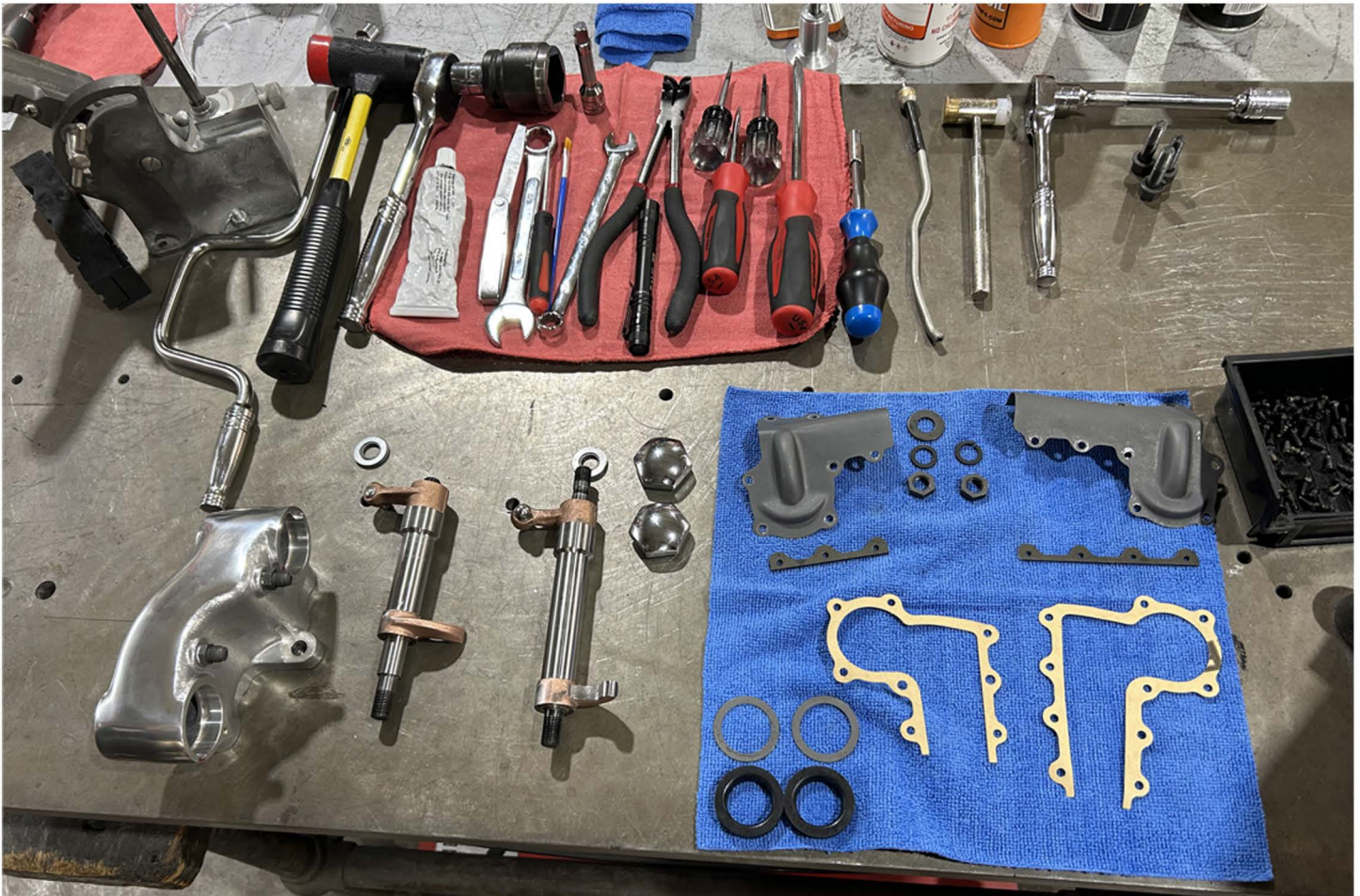
Basic front cylinder head component layout
