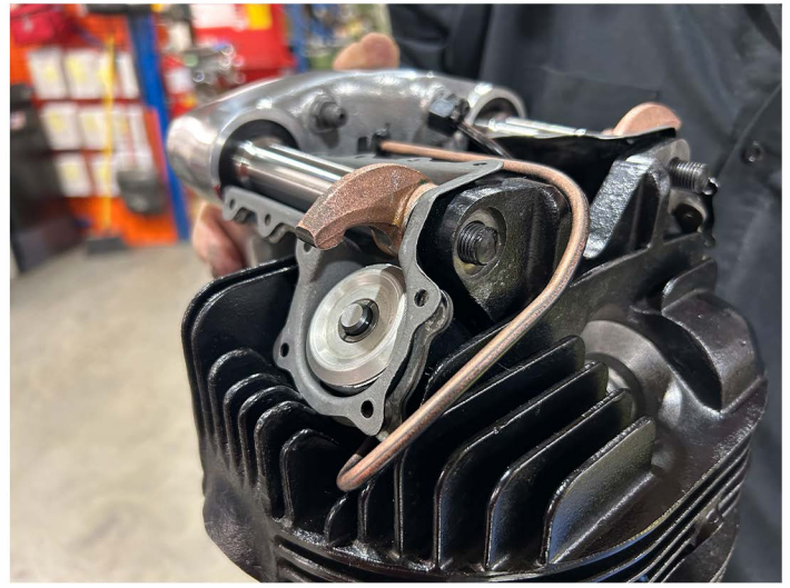
Rocker Box assembly ready to receive each respective shaft hardware.
