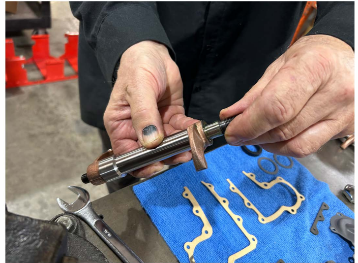
Insert Rocker Shaft into Rocker Arm itself.
